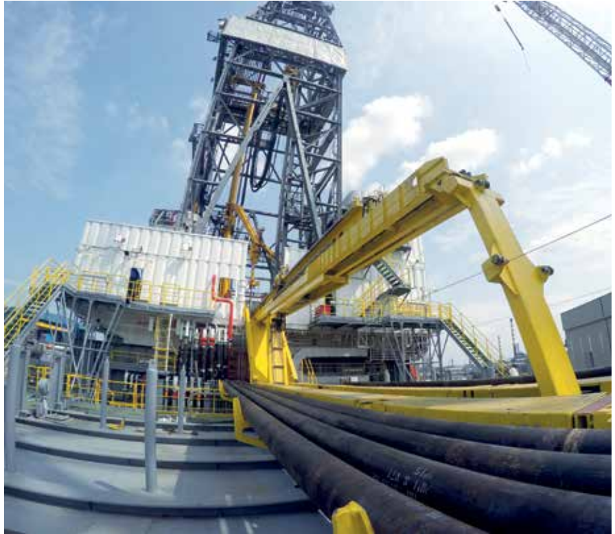
The hydraulic catwalk (pictured) installed on a KFELS B Class jackup rig offers best-in-class cycle times for moving drill pipes and tubulars from the pipe storage area up to the drill floor
